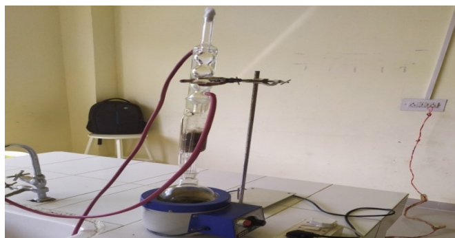
Figure 2: Assembly of Soxhlet extraction apparatus
